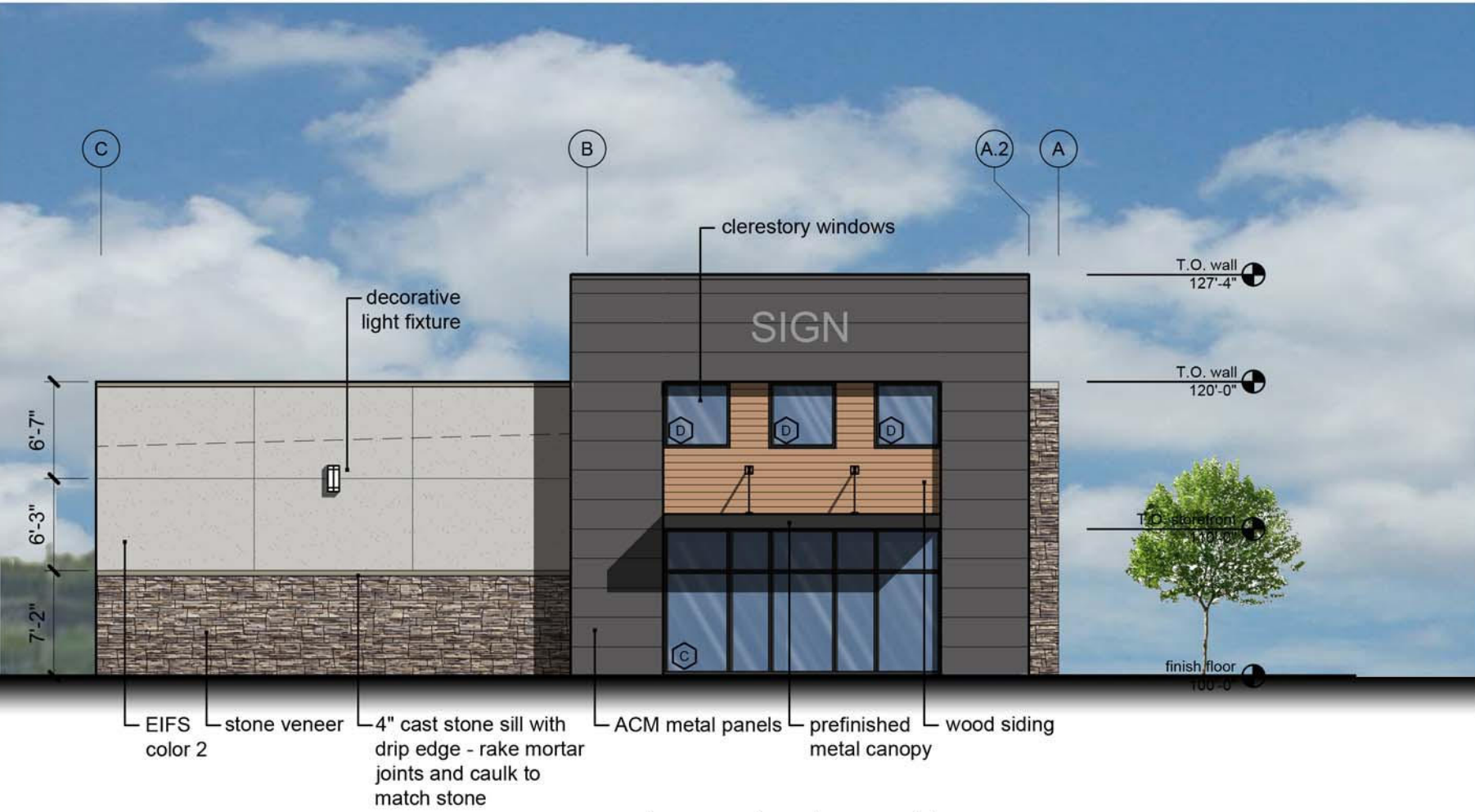
2 east elevation scale: 3/32"=1'-0"
