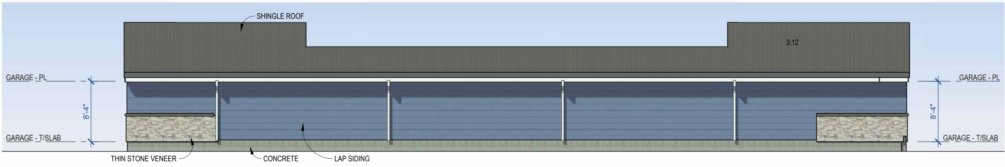
TYPICAL DETACHED GARAGE REAR ELEVATION 1/8" = 1'-0"
