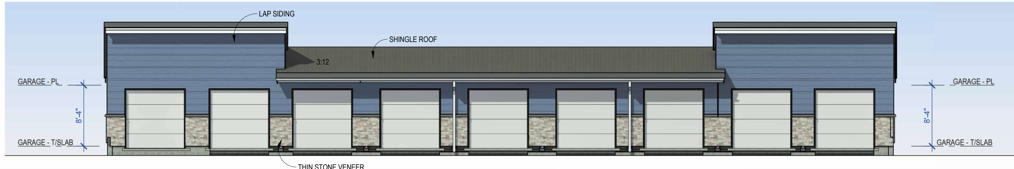
TYPICAL DETACHED GARAGE REAR ELEVATION 1/8" = 1'-0"
